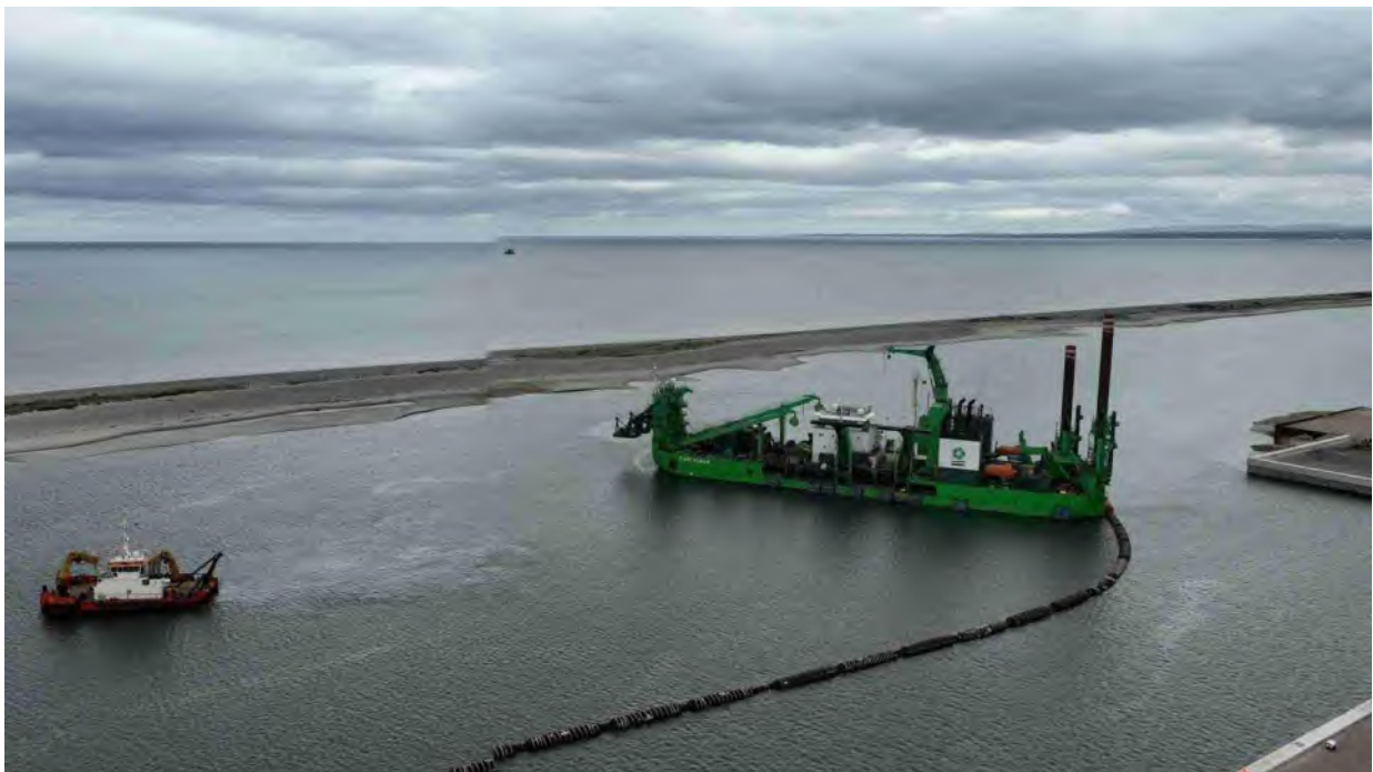
Image 3.2: Picture of a Cutter Suction Dredger
