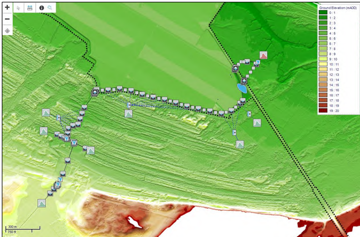
Figure 6.1: Eastern Watercourse 1D model schematic, with LiDAR-based ground elevations (external to site) and proposed platform elevations (within the site)
